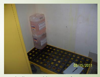
The secondary containment on the left is very shallow and is meant for use only with small containers. Use this style with caution, it is easy to put too large a container on it.
